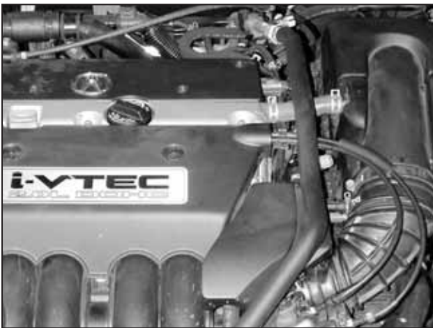
Factory air box system installed
