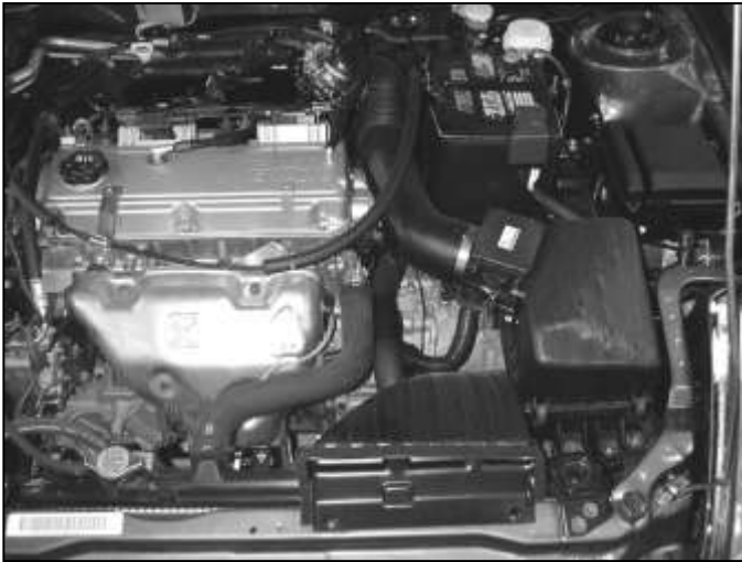
Factory air box system installed
