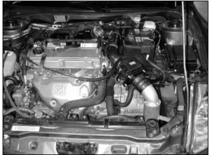
AEM® intake system installed
