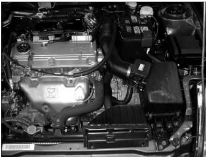
a. Factory air box system installed.
