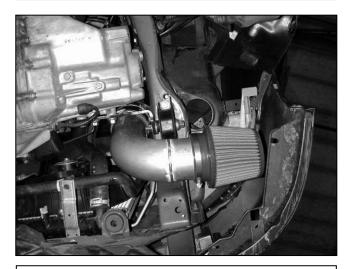
i. Install the AEM<sup>®</sup> air filter onto the short leg of the lower intake pipe. Then attach the lower pipe assembly to the upper intake pipe using the supplied coupler and hose clamps. Position the assembly so the air filter has adequate clearance.
