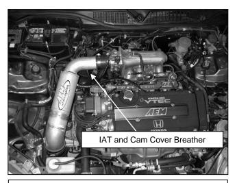
g. Install the intake pipe using the included coupler and #44 clamps. Install the IAT sensor in the rubber grommet. Also install the 3/8" hose on the intake pipe and the cam cover breather nipples.
