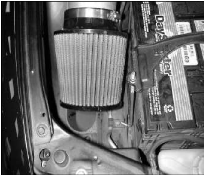
i. Next install the AEM ® filter on to the end of the inlet tube. Push the air filter over the inlet pipe until it mates to the step inside the air filter inlet. Install the supplied #64 hose clamp to secure the filter onto the inlet pipe. Tighten the hose clamp after this is done.
