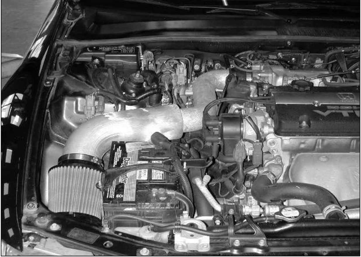
j. Check that the air filter is not touching any part of the vehicle. Position the inlet pipe for best fitment. Be sure that the pipe or any other component is not in contact with any part of the vehicle. Tighten the hose clamps at the throttle body. Tighten the nut on the rubber mount. Check for proper hood clearance. Readjust pipe if necessary.
