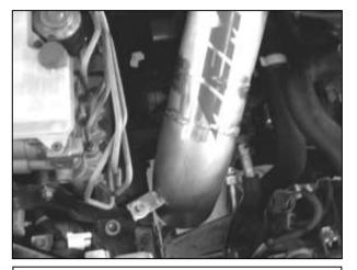
e. Align the tab on the intake pipe with the rubber mount. Install the 6mm nut and washer according to the diagram below. Do not tighten the nut.
