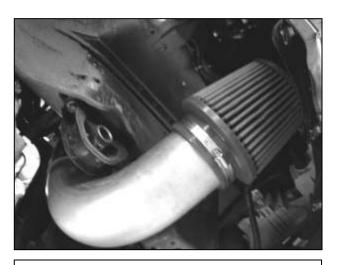
g. Install the air filter on the long end of the 4" diameter elbow. Install the 4" silicone coupler on the short end of the pipe. From underneath the vehicle, place the other end of the coupler on the end of the upper intake pipe as shown in the picture. Position the assembly so that no part of the pipe touches the vehicle.
