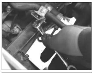
i. Using the M6 x 15mm bolt from the AEM® kit, bolt the spacer to the bracket.
