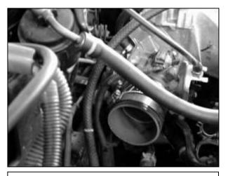
c. Insert the 2.75" silicone coupler on to the throttle body. Place two #44 hose clamps on the coupler but do not tighten yet.
