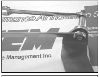
c. Install the factory mounting stud from step 3b on the supplied engine mount bracket, using the nylock nut and washer provided.
