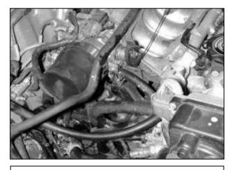
c. Insert the 2.5" x 3.0" coupler onto the throttle body (this is a tight fit). Slide the two #44 hose clamps over the end of the coupler.
