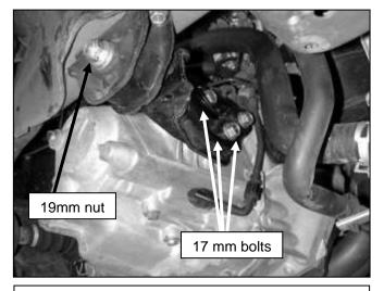
a. Using a 19mm socket, remove the engine mount nut, then loosen the three bolts with a 17mm wrench, and remove the mount.
