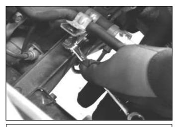
g. Using the M6 x 15mm bolt from the  $AEM^{(B)}$  kit, bolt the spacer to the bracket.
