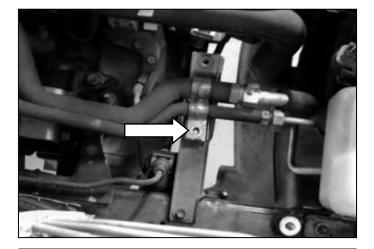
e. Remove the bolt holding the A/C line bracket in place.
