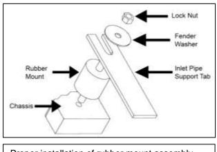
Proper installation of rubber mount assembly.
