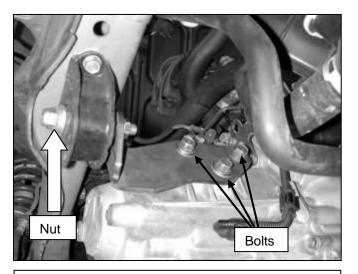
d. Using the supplied bolts and the factory washers, install the AEM<sup>®</sup> engine mount on the transmission, then replace the factory washer and nut on the mounting stud.
