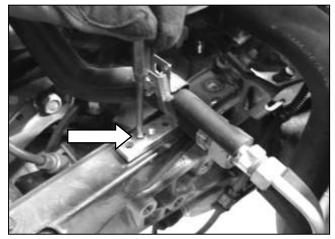
f. Install the spacer from the AEM<sup>®</sup> kit in place where the A/C line bracket was bolted. Install it with the pin inserted into small un-threaded hole on the bracket. It may be necessary to push the pin into the hole with a punch or similar tool. Make sure that the spacer is oriented with the threaded hole toward the A/C lines.
