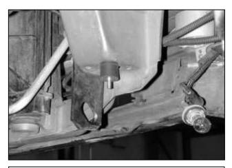
b. Install the rubber mount in the hole on the underside of the frame next to the frame hook as shown in the picture.
