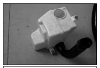
d. Remove the resonator from the cavity behind the front bumper (older models will be black).
