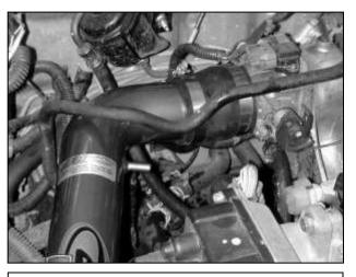
g. Install the 3/8" hose from the valve cover vent to the nipple on the intake pipe. Secure it in place with 3/4" hose clamps.
