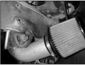
h. Install the air filter on the end of the intake pipe. Make sure the air filter is fully seated on the end of the pipe. Secure it in place with the supplied hose clamp.
