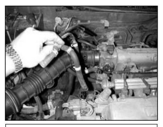
c. Detach the PCV hose from the fitting on the valve cover. Remove the hose assembly from
