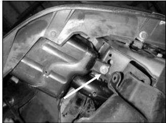
j. Remove the three bolts holding on the air intake resonator assembly and remove it from the vehicle.
