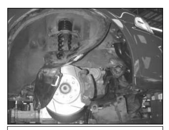
i. Tuck the fender liner out of the way behind the brake rotor.
