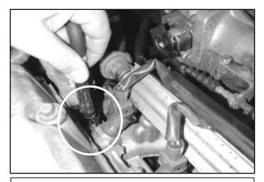
a. Remove the water hose on the left of injector #4 by loosening the hose clamp and sliding the water hose upward. Be prepared to catch any coolant that spills out with a rag.
