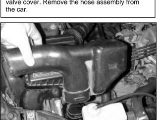
e. Remove the air intake snorkel by pulling it straight up until it unsnaps.
