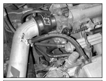
g. Insert the 2.5" end of the pipe into the silicone coupler on the throttle body. Use the #40 hose clamps on the coupler. Install the 3/8" ID hose from the valve cover breather fitting to the nipple on the intake pipe. Use the 1" hose clamps to secure it in place.
