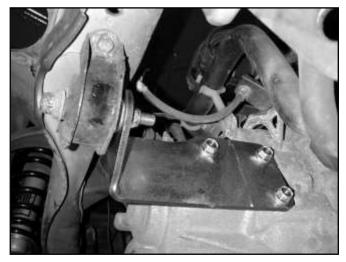
d. Using the supplied bolts, install the  $\mathsf{AEM}^{\$}$  engine mount on the transmission; torque the bolts to 61 ft-lb. Then replace the factory washer and nut on the mounting stud.
