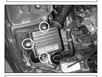
f. Remove the three air box mounting bolts and remove the factory air intake system from the car.
