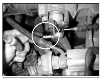
b. Remove the other end of the water hose from the fitting underneath the throttle body.
