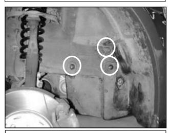
g. After removing the front right wheel, remove the fender liner fasteners shown in the picture.
