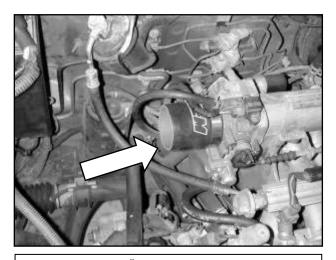
c. Install the  $\mathsf{AEM}^{\texttt{@}}$  silicone coupler onto the throttle body.
