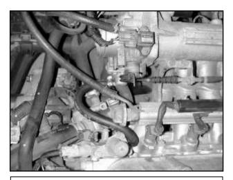
b. Install the 5/16" ID hose, and two 3/4" hose clamps, in place of the hose assembly removed in Section 2a & 2b.
