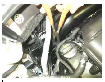
b. Disengage the spring clamp retaining the coupler on the turbo inlet.
