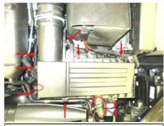
a. Fully loosen the 8 screws on the top of the air box. Pull off the hose on the left & disconnect the hose on the front of the air box to access & replace the OE filter with the filter provided in this kit. Reinstall screws and hoses.
