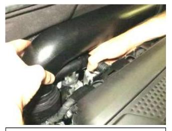
e. Lift the coupler and hose assembly off the turbo inlet to access the PCV hose. Disconnect it by pulling firmly straight off. Remove the hose assembly from the vehicle.
