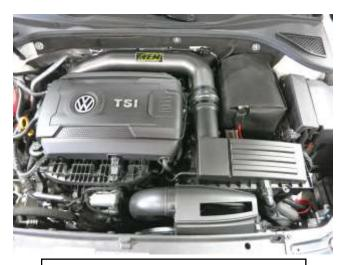
g. Finished installation of AEM Intake System.
