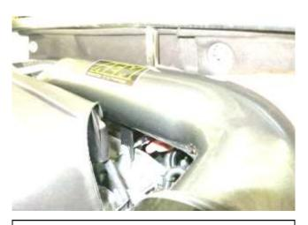
d. Reinstall the tube mounting bolt taking care to position your new intake tube with clearance all around.
