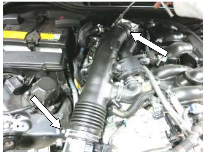
d. Loosen the stock hose clamps on both ends of the intake tube using a 10mm socket and remove the tube.
