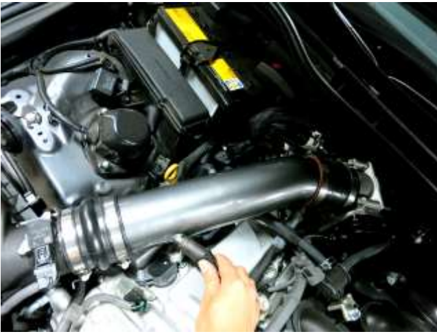
e. Reconnect the breather hose to the AEM tube.
