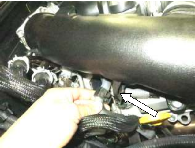
c. Detach the vacuum line harness from the intake tube as shown.
