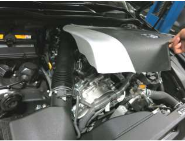
a. Lift up the engine cover and set aside.
