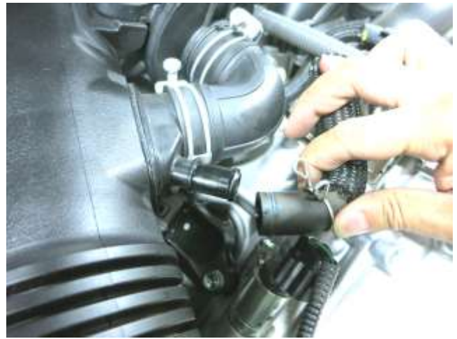
b. Disconnect the breather hose from the stock intake tube.
