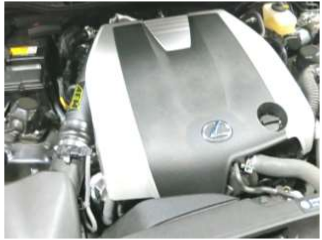
f. Reinstall the engine cover. Check for clearance between the tube, engine, and engine cover prior to fastening all hose clamps.
