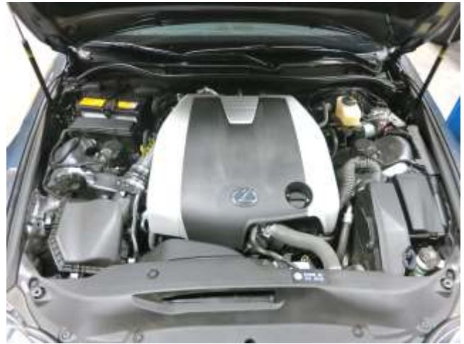
h. Finished installation of AEM Intake System.
