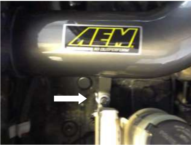
g. Install the intake tube into the accelerator first then, slide the coupler over the air box inlet. The bracket should line up to the rubber mount as well.
