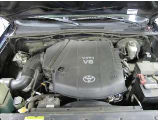
Factory air box system installed
