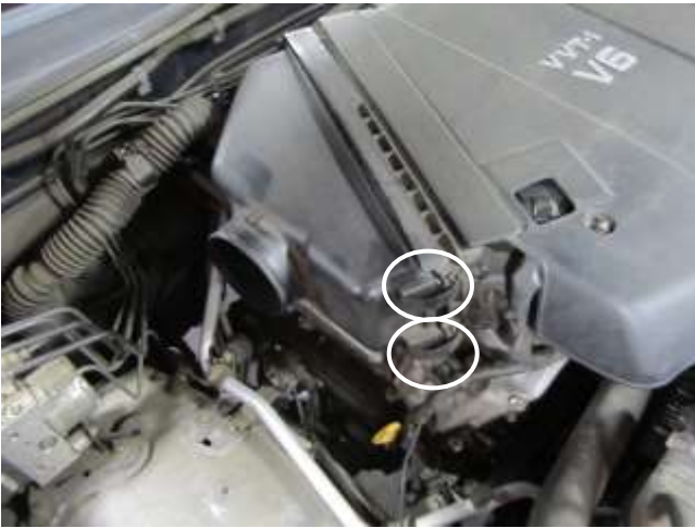
c. Attach the clips that were undone in step 2d.
