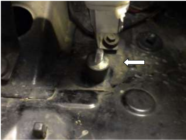
d. Install the supplied rubber mount into the threaded hole next to the reservoir as shown.
