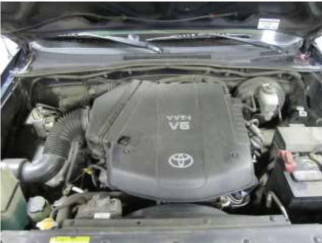
Factory air box system installed
