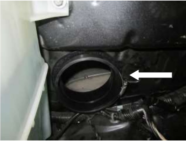
e. Install the edge trim (8-4108) onto the fender. Then squeeze the air accelerator while installing it into the fender with the flat side of the horn pointing down and slide hose clamp on.
