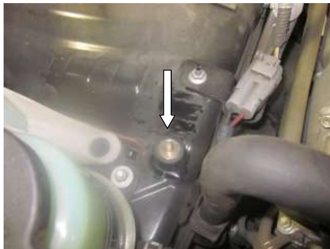
b. Install the provided (1228560) mount into the body of the vehicle where the M6 bolt was removed in 2e.
