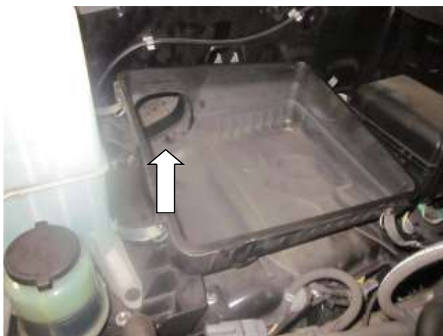
c. Install the lower air box into the vehicle by squeezing the air accelerator and inserting it into the fender opening in the vehicle. Note: it 's easier to have the air box lid and base separated to perform this step.
