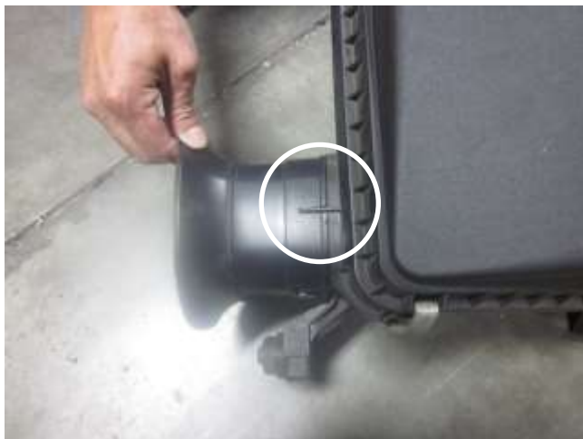
a. Install the AEM air accelerator onto the air box by aligning the slot in the box and the air horn.
