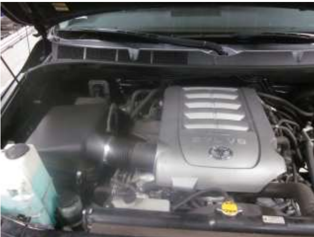
Factory air box system installed
