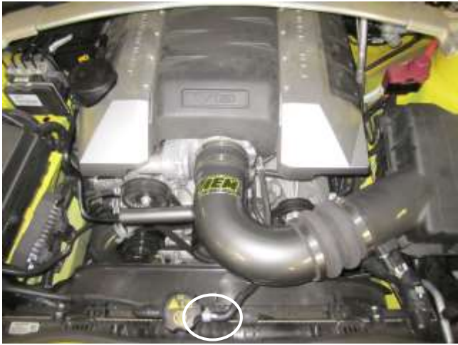
f. Install the other end of the intake tube into the hump hose coupler. Note: Due to factory tolerances, the coolant recovery hose may need to be adjusted to not interfere with intake tube.
