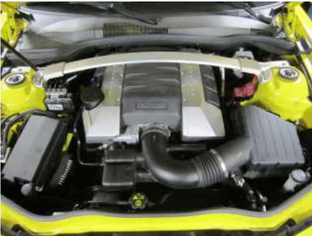
Factory air box system installed
