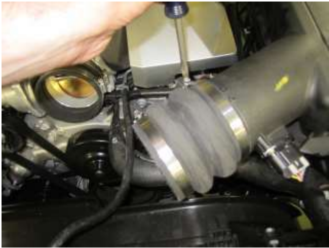
d. Install the hump hose (5-1090) with the two supplied hose clamps (9464) onto the air box inlet. Note: Some mild soap and water mixture may be used to ease installation .
