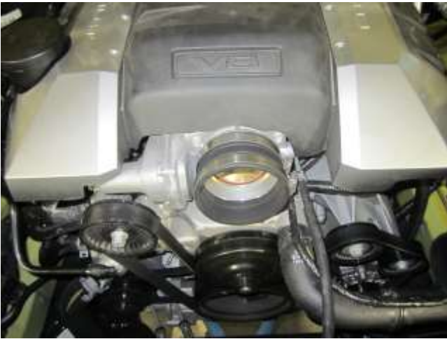
c. Install the coupler (341018) with the two provided hose clamps onto the throttle body. 9460 goes on the throttle body, 9464 goes on the AEM Intake tube.
