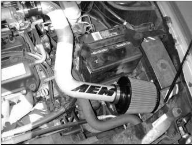
AEM® intake system installed
