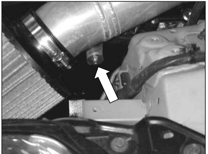
o. Align the mounting bracket to the rubber mount installed in step 3b. See diagram below for proper assembly.
