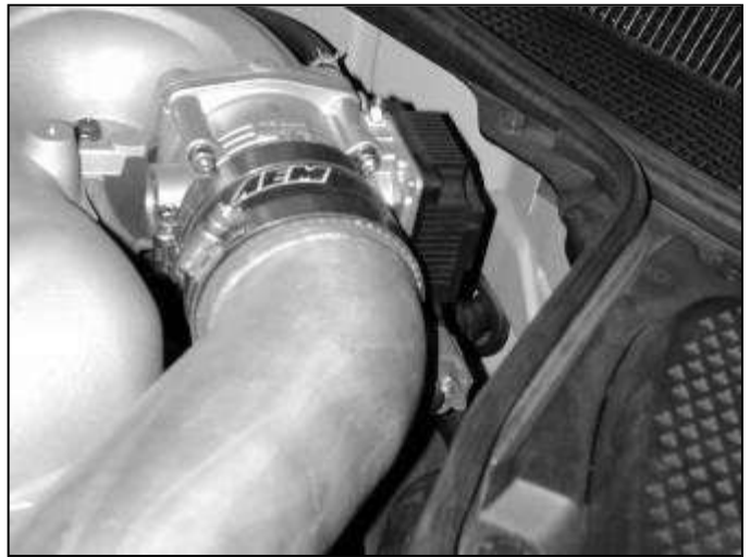
m. Insert the inlet pipe into the coupler. The bracket should be on the opposite side.
