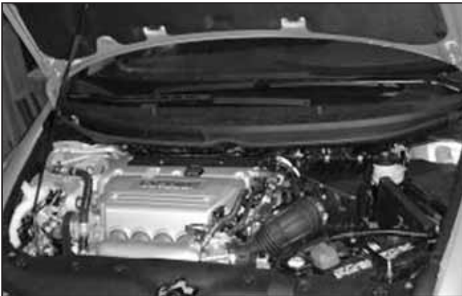
Factory air box system installed
