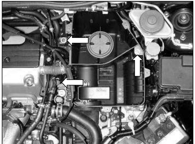
d. Loosen the 3 bolts holding the air filter assembly, and remove it.
