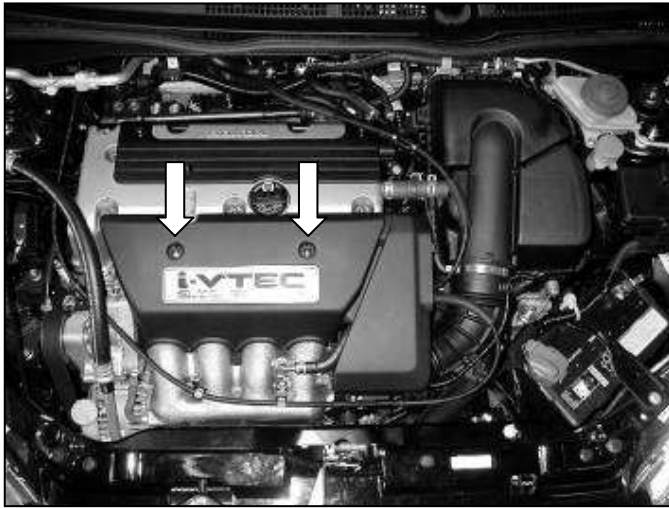
a. Loosen the two bolts holding the intake cover, then remove it.
