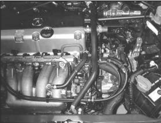
l. Factory air box system removed from the vehicle.
