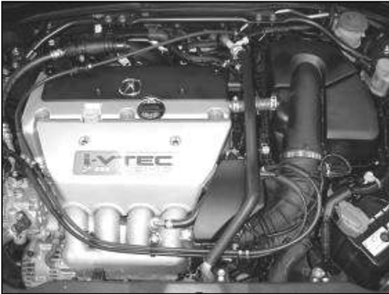
a. Factory air box system installed in the vehicle.
