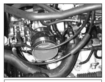
c. Install the included rubber reducer coupler onto the throttle body using the supplied No. 44 clamp, and place the No. 48 clamp over the large end of the coupler.
