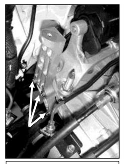
f. Loosen the three 10mm bolts, and remove the air filter box mount.
