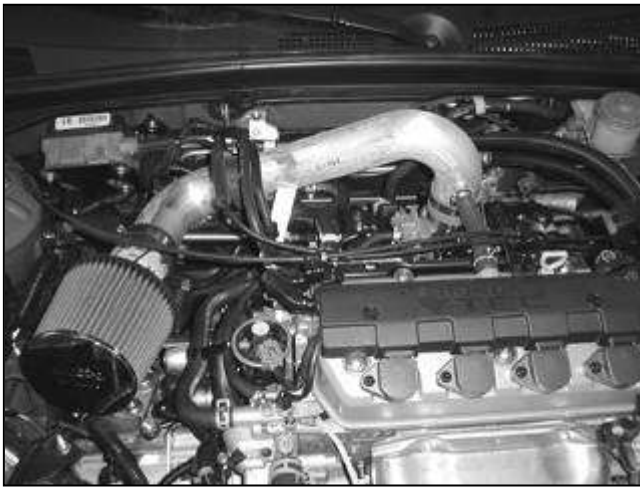
AEM® intake system installed
