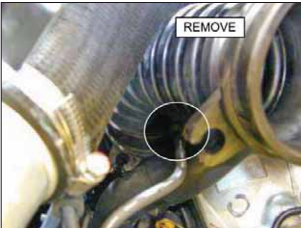
k. Disconnect vacuum line from the boost solenoid to the turbo inlet hose. The vacuum line is located underneath the turbo inlet hose. Remove the turbo inlet hose.
