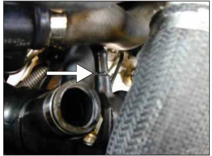
j. Disconnect the crankcase breather tube at the turbo inlet hose.
