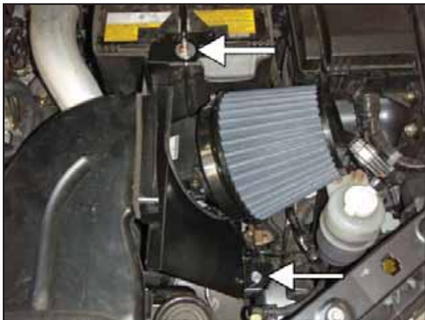
r. Insert heat shield. Align with the battery bracket and secure with a washer and factory nut. Secure the other mounting point of the heat shield with the provided bolt.
