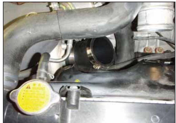
c. Attached assembled coupler to the turbo inlet as shown.
