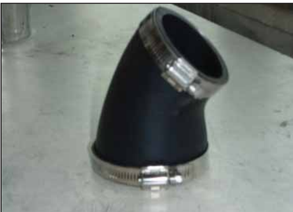
b. Assemble the 45 degree coupler as shown with hose clamps attached loosely.
