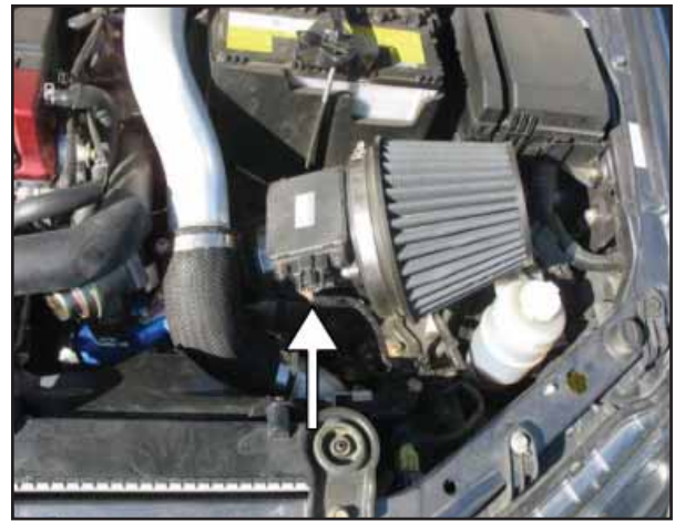
p. Reattach MAF sensor harness. Some vehicles may require that you remove approximately 2" of wire loom tape to create more slack to route the MAF harness.
