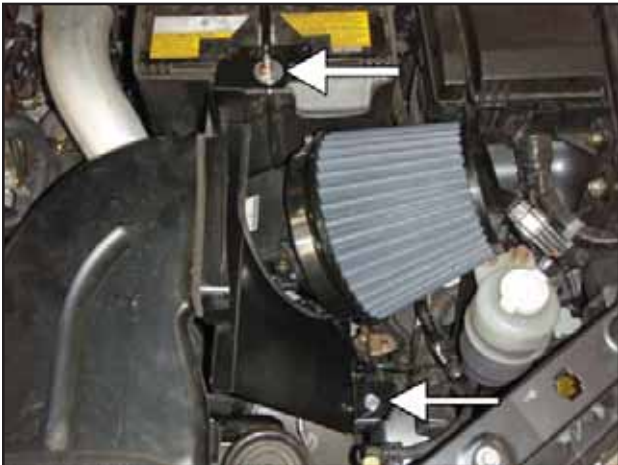
r. Insert heat shield. Align with the battery bracket and secure with a washer and factory nut. Secure the other mounting point of the heat shield with the provided bolt.
