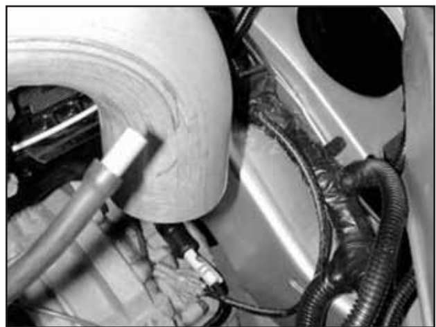
n. Attach vacuum fitting to the other end of the vacuum line.
