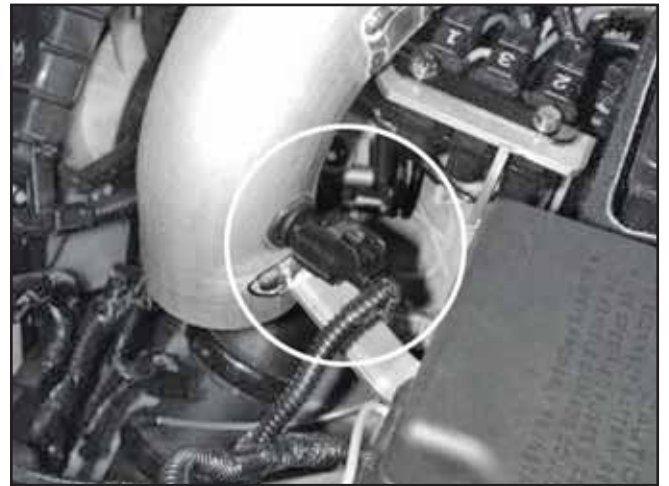
l. Reinsert IAT sensor into the rubber grommet.
