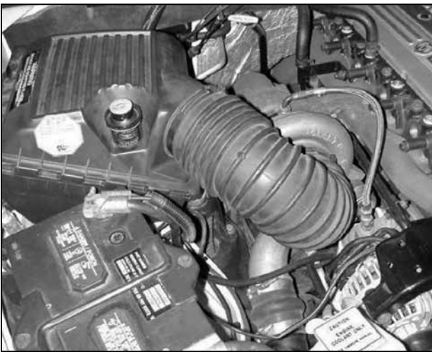
Factory air box installed
