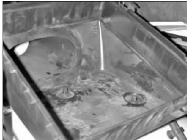
d. Remove the snorkel from the lower air filter housing by squeezing the middle together while pulling towards the center of the vehicle.
