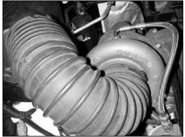
b. Loosen the hose clamps securing the flexible inlet hose between the turbo inlet and the air filter housing. Remove the flexible inlet hose.
