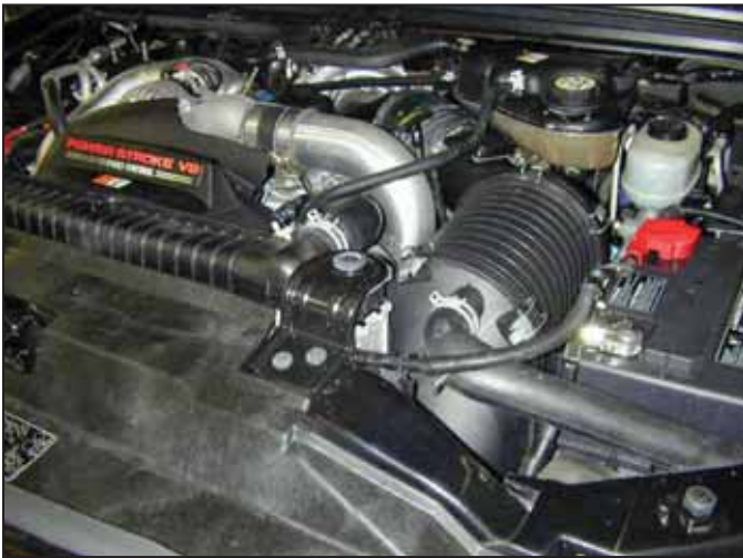
Factory air box system installed
