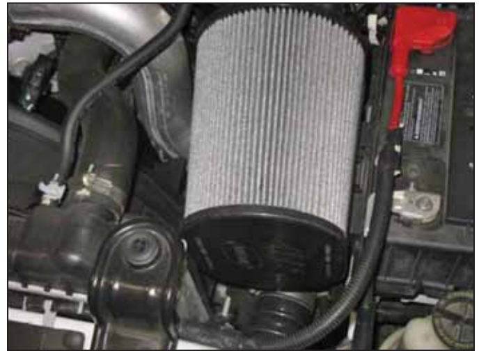
AEM® intake system installed
