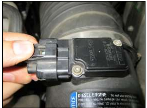
B. Depress the snap tab on the MAF sensor connector as shown and pull it to disconnect the harness from the sensor.
