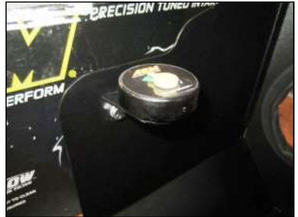
F. Install the AEM® Filter Minder™ Gauge (N) into the mounting grommet as shown. Use glass cleaner or silicone spray lubricant to lubricate the grommet and completely seat the gauge.
