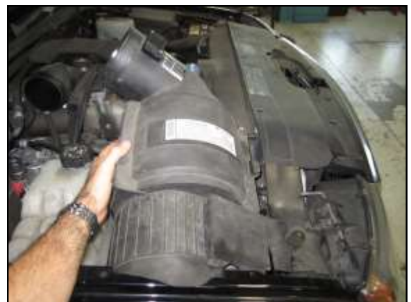
D. Pull up on the stock filter air box starting on the side closer to the engine to "pop" it free from the 3 mounting grommets. Remove the air box assembly from the engine bay.
