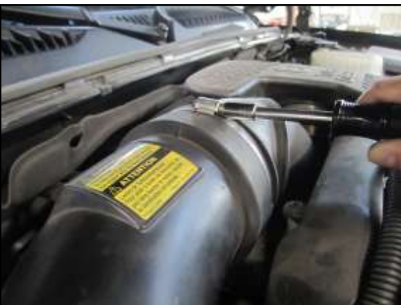
C. Loosen the two hose clamps retaining the stock intake tube at both ends and remove the tube from the engine bay.
