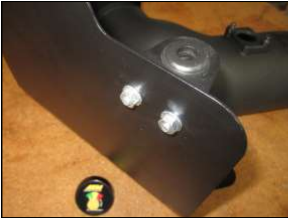
E. View of the M6 nuts (U) on the outside of the heat shield to mount the bracket.
