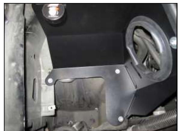
J. Install the AEM® heat shield into the engine bay using 3 of the stock M6 bolts with washers from the stock mounting plate as shown and tighten the bolts.
