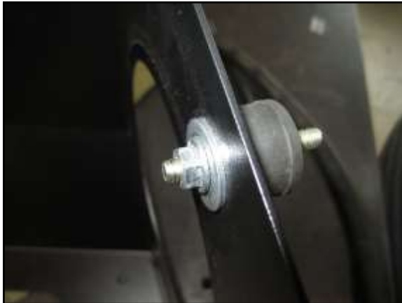
G. Install the M6 rubber isolator mount (K) into the hole over the large opening in the heat shield (B), then install one flat washer (X) and one M6 nut (U) on the inside of the heat shield as shown. Tighten the nut.
