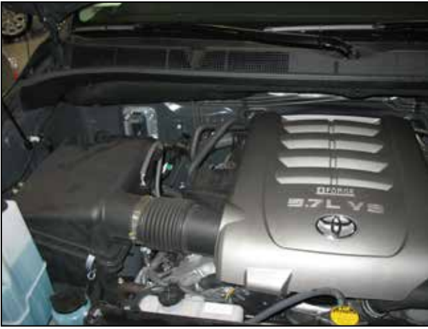
Factory airbox system installed
