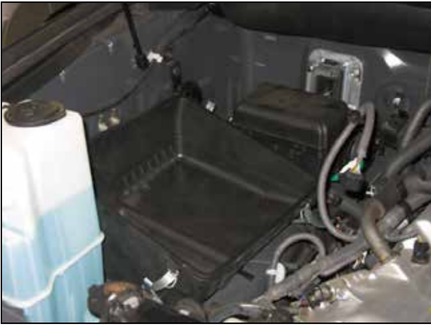
k. Remove the stock air filter from the lower airbox.
