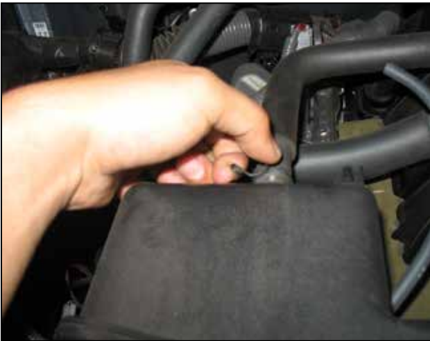
c. Pinch the hose clamp, and remove the larger hose from the inlet resonator.
