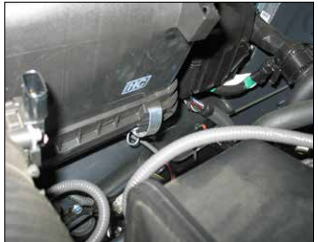
h. Unclip the forth airbox clip.
