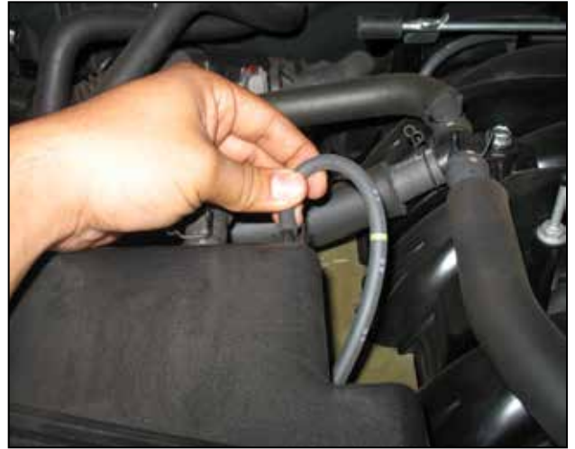
b. Remove the small hose located on the back of the inlet resonator.
