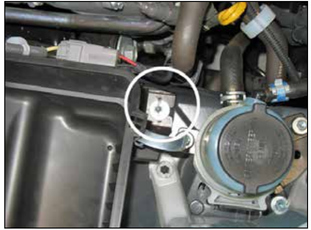
l. Unscrew the two bolts that secure the lower airbox. The location of the first bolt is pictured above.
