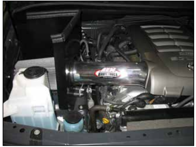
AEM® intake system installed
