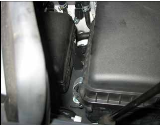
g . Unclip the third airbox clip.
