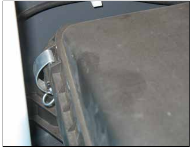
f. Unclip the second airbox clip.
