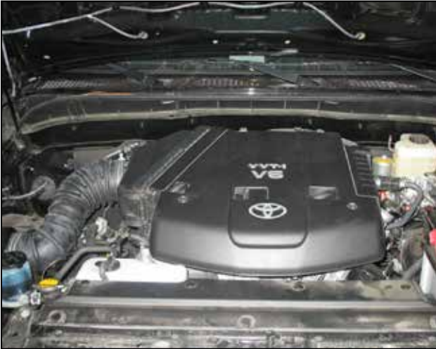
a. Factory air box system installed.
