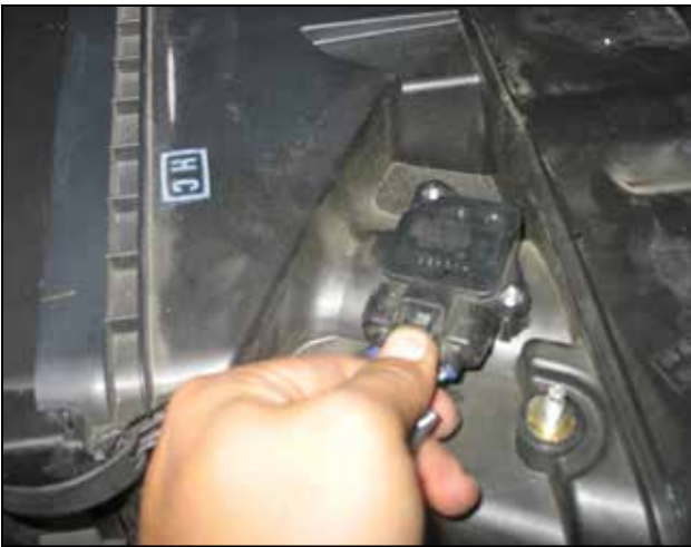
c. Disconnect the wire harness connector from the mass air flow (MAF) sensor.
