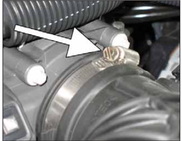
b. Loosen the hose clamp securing the inlet tube to the throttle body.
