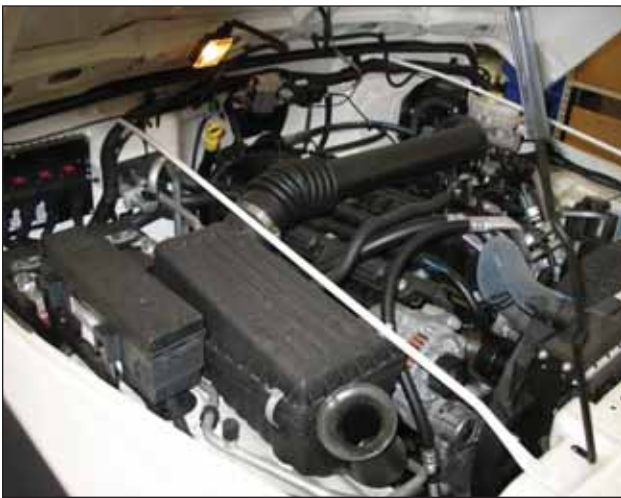
Factory air box system installed
