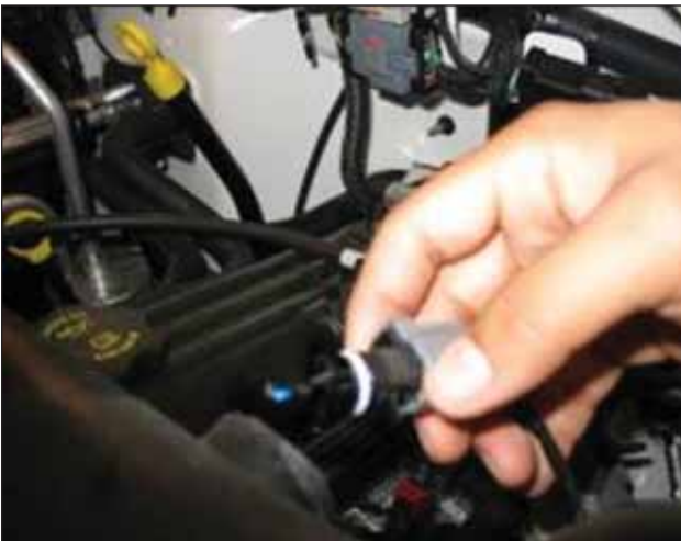
c. 2005-2006 Vehicles: Push in and twist the "Inlet Air Temperature" sensor out of the intake tube. 1997-2004 Vehicles: Proceed to the next step and disregard this step.
