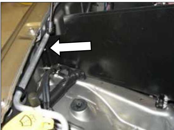
h. Insert the heat shield. Secure with the provided washers and nuts. Check for factory installed hardware. If studs are secured with nuts already, remove first. Use care to avoid damaging the vacuum hoses or the wire harness.
