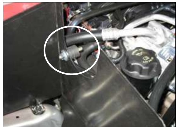
i. Attach the rubber mount and secure with 8mm washer and nut.
