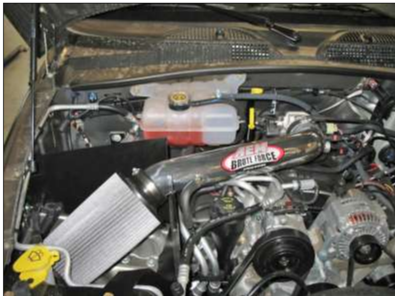
AEM® intake system installed
