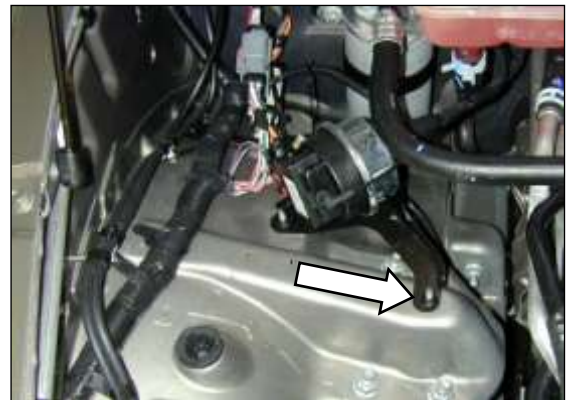
g. Loosen and remove the mounting nut. This nut will be reused if your vehicle has cruise control. If your vehicle is not equipped with cruise control, then use the provided M6 nut.
