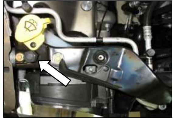
e. Remove the bolt, it will be reused in a later step.
