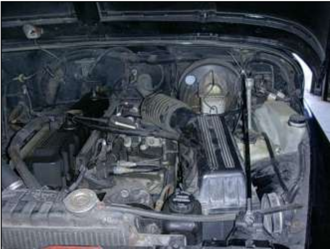
Factory air box system installed
