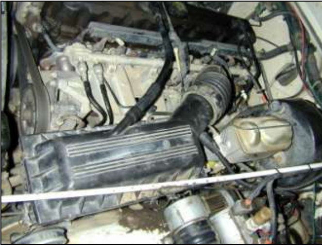
a. Factory air box system installed.
