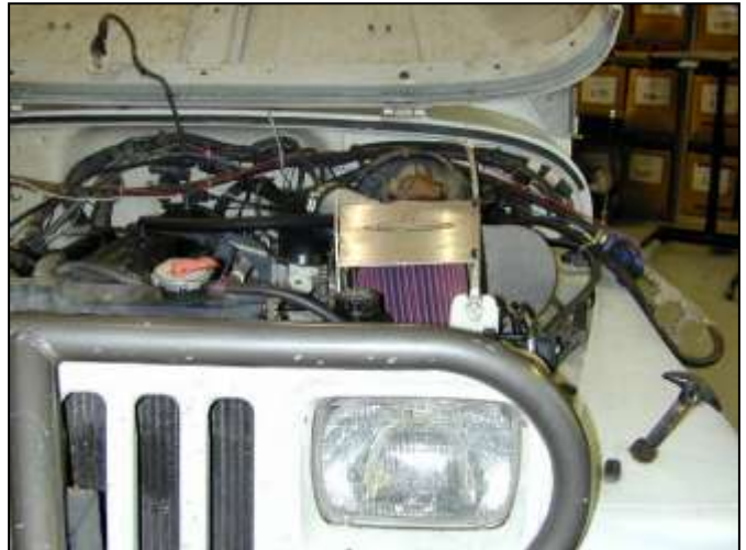
AEM ® intake system installed
