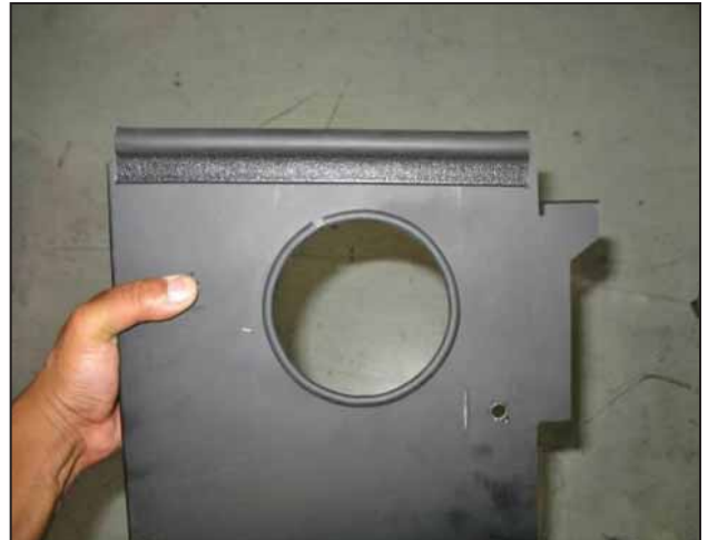
c. Attach the foam gasket onto the top of the heat shield.
