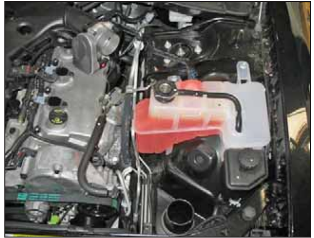
f. Remove the air box assembly from the engine bay.
