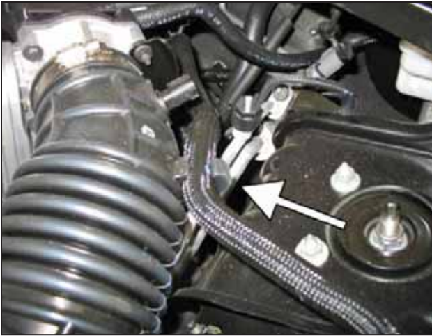
e. Remove the coolant line from the air tube.
