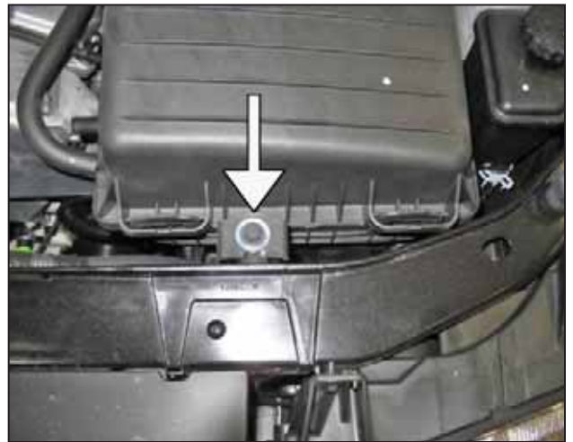
d. Loosen and remove the air box mounting screw. This screw will be reused.
