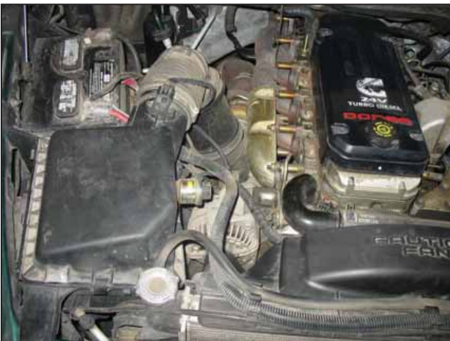
Factory air box system installed
