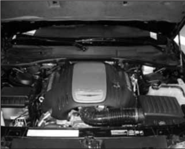
a. Factory air box system installed.
