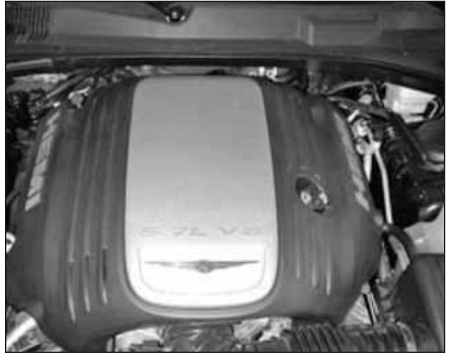
b. Remove the engine cover by pulling straight up.
