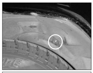
d. From the wheel-well side of the inner fender, secure the rubber mount in place with a fender washer and lock nut.
