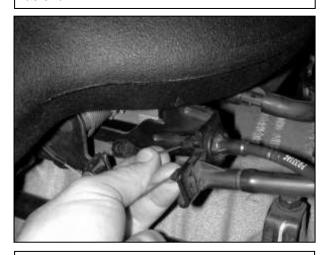
I. Re-attach the cable to the bracket on the throttle body. Snap the end of the cable back on to the throttle linkage control arm. Plug the vacuum line back on to the connector on the firewall.
