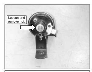
c. Loosen and remove mounting nut and washer.
