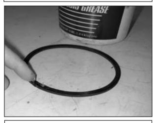
e. Apply a very thin coat of grease to both sides of the circular rubber gasket included in the kit.
