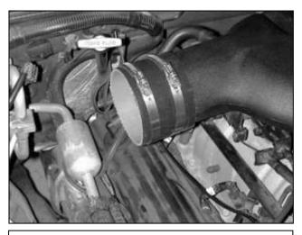
j. Install the silicone coupler on to the end of the upper intake plenum.
