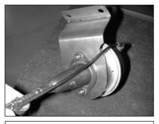
j. Install the cruise control cable cover and secure it in place by re-using the factory nuts. Make sure the vacuum hose fits in the cut-out as shown.
