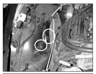
b. Remove the plastic fastener holding the inner fender liner in place, as seen in the picture. Unscrew the factory air box mount from the stud on the inner fender.
