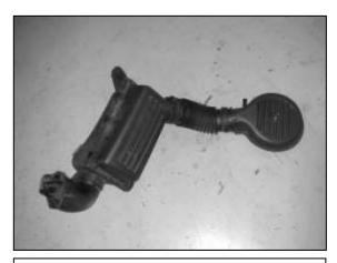
c. Remove the factory air inlet system from the vehicle.
