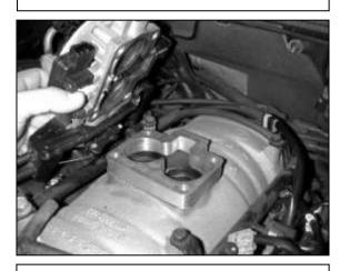
d. Lift up the throttle body and remove the factory gasket. Place the AEM® throttle body spacer on the intake manifold. Use the supplied new gaskets on each side of the spacer. Make sure the spacer is oriented correctly.
