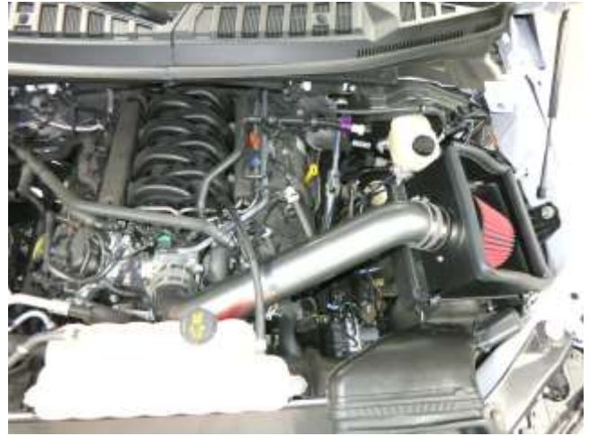
p. Finished installation of AEM Intake System.
