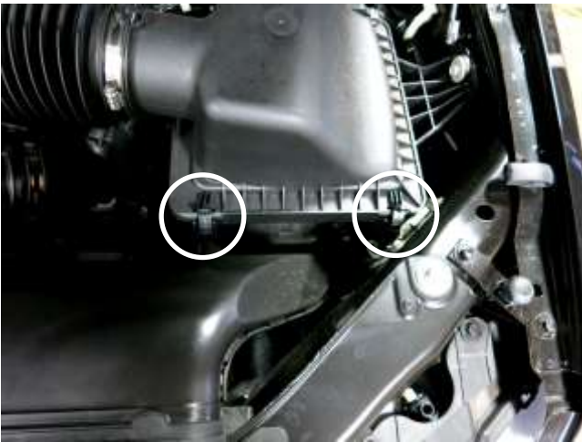
a. Detach the two latches securing the upper air box lid to the lower air box lid.
