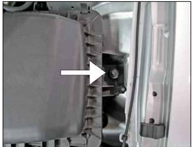
d. Loosen and remove the M6 bolt securing the airbox to the inner fender.
