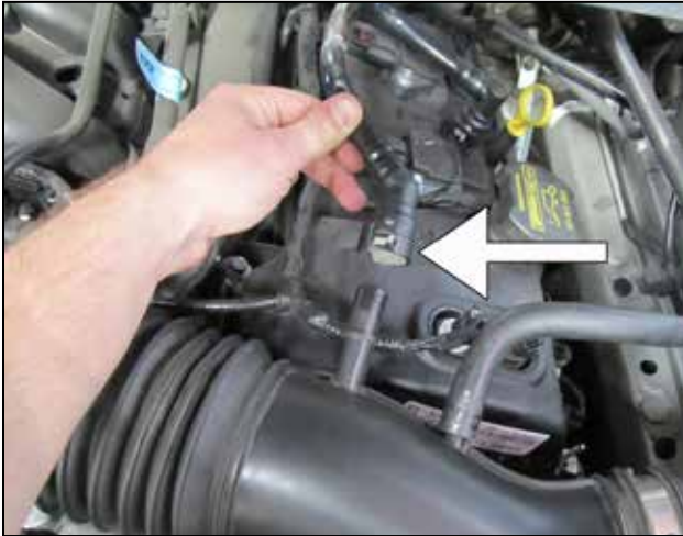
a. Disconnect the crankcase vent line.
