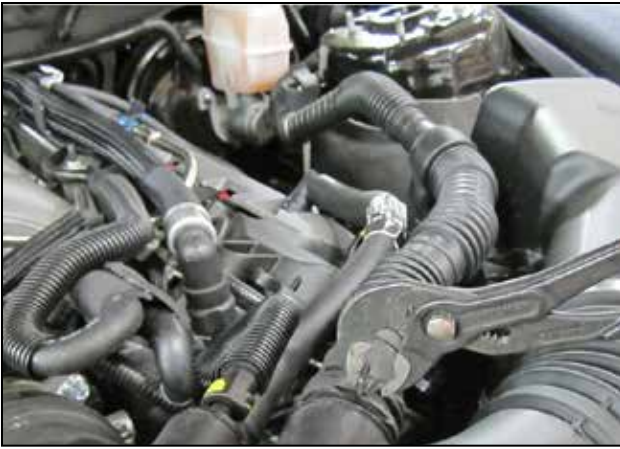
e. Release the spring clamp on the sound tube using a pair of pliers.
