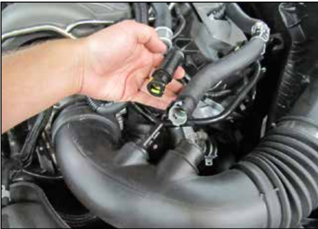
g. Release the crankcase vent tube from the nipple. Slide the gray clip to the side and pull on the connector to release it. On auto. trans. vehicles, also release the smaller vent tube by squeezing the yellow clip.
