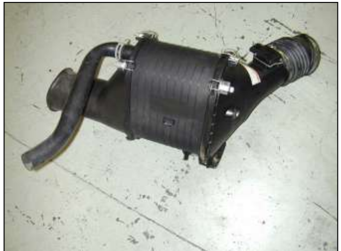
h. Remove the remaining stock air box system.
