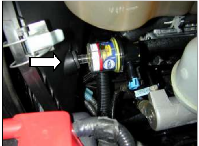
f. Pull the air filter status meter from the grommet.
