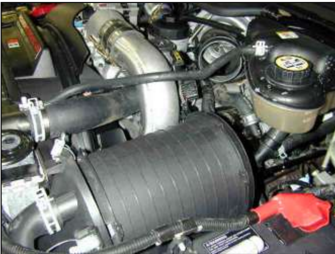
g. Remove the rear section of the intake system.
