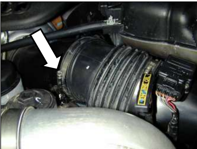
c. Loosen the hose clamp on the turbo inlet pipe.
