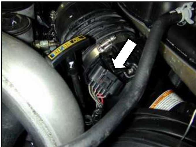
d. Vehicle equipped with MAF sensor. Unplug the mass air flow (MAF) sensor.
