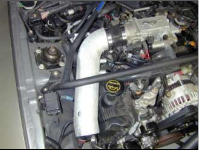
c. Insert inlet pipe into coupler. Do not completely tighten hose clamp.
