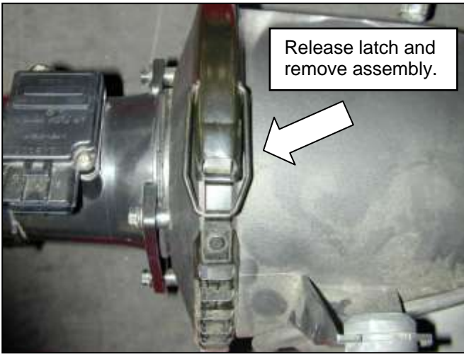
e. Release latch and remove the air filter element and housing.
