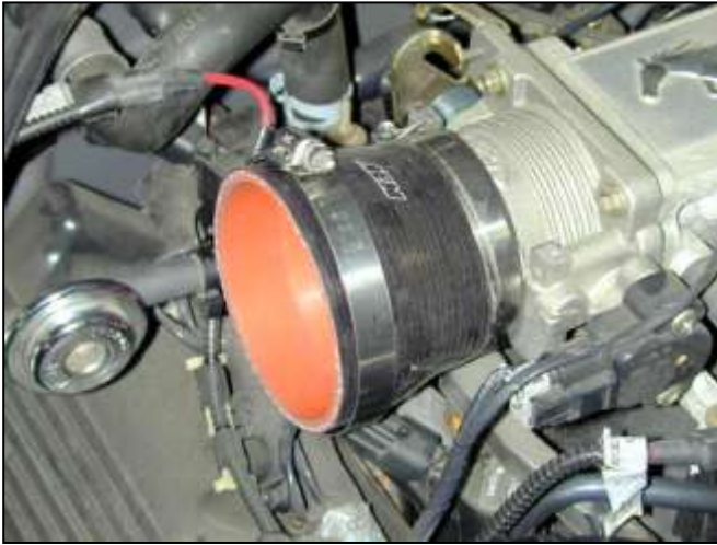
b. Attach reducer coupler and hose clamps. Do not completely tighten.
