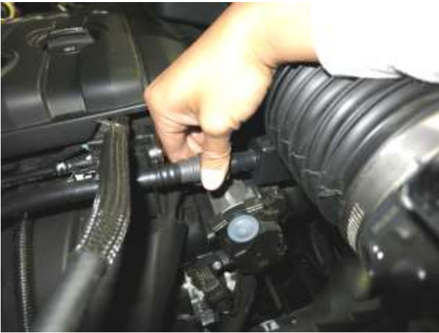
e. Disconnect the breather hose located at the rear of the stock intake tube.
