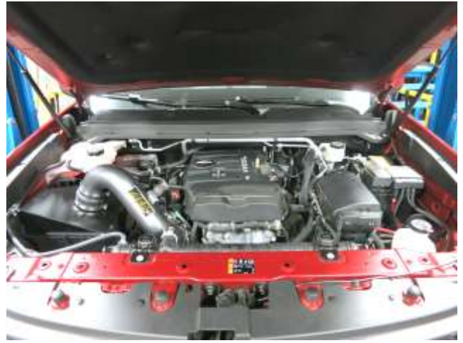
l. Finished installation of AEM Intake System.
