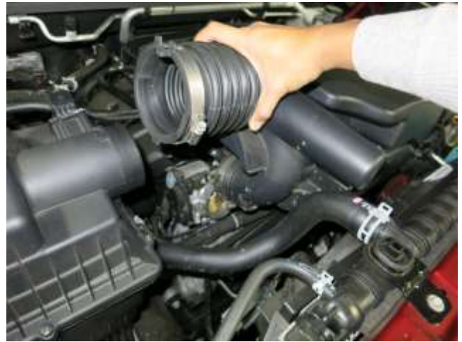
f. Slide the couplers off the airbox lid and throttle to remove the upper resonator assembly.
