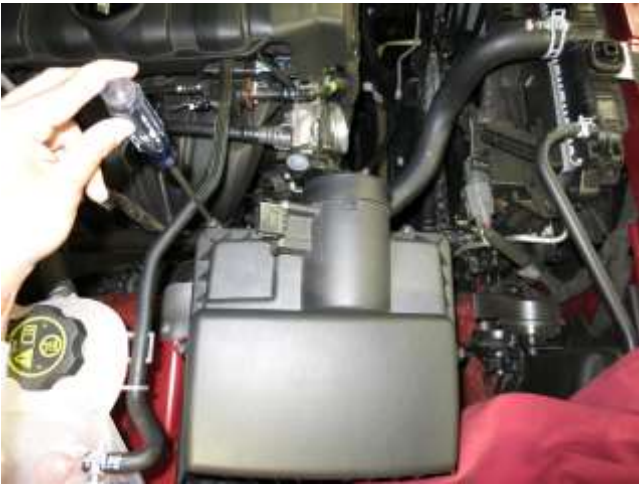
g. Use a Phillips screwdriver to remove the 4 screws securing the airbox lid to its base.
