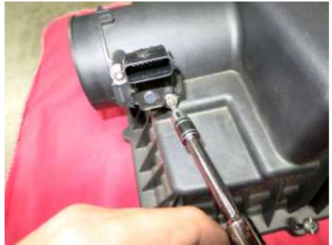
h. Use a T20 Torx bit to remove the MAF sensor from the airbox lid.
