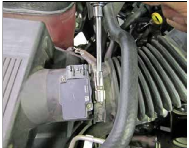
d. Loosen the hose clamp that secures the inlet tube to the air filter box.
