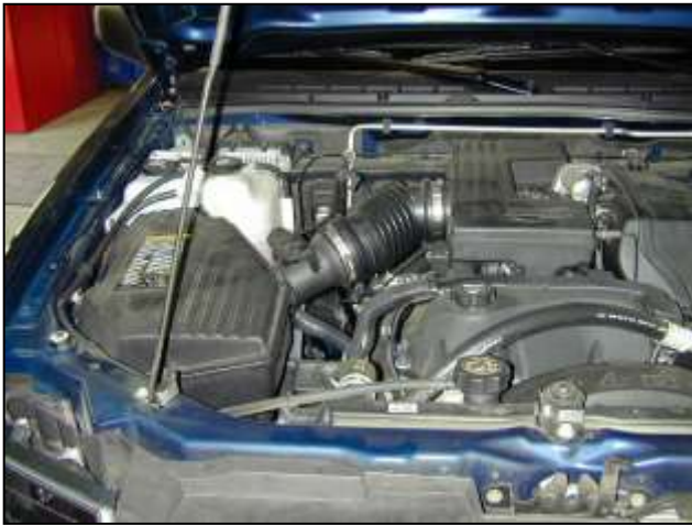
a. Factory air box system installed.
