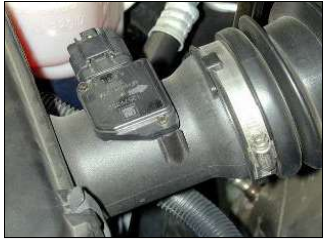
b. Unplug the wire harness from the Mass Air Flow (MAF) sensor. Remove the two screws retaining the MAF sensor and carefully remove the MAF sensor.
