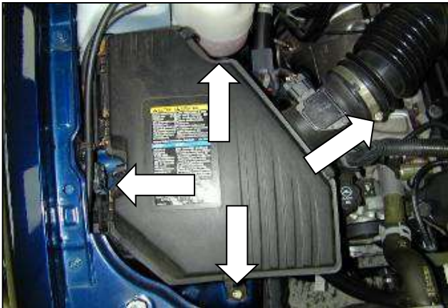
c. Loosen the hose clamp on the stock air box. Remove the air box by removing the two bolts and the nut securing it. Lift air box out of vehicle.
