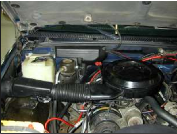
Factory air box system installed
